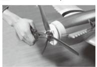
10 Install the propeller.
